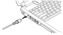
Figure B-2.Connecting the Antenna
